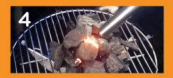
Push the Rear Main Control switch to activate the blower. Aim the airflow at the ignited area to spread the heat until your fire is strong. The closer you hold the barrel to your wood or coals, the faster your fire will spread.
