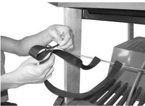
Slide the loops of the Gas Bottle Strap (21) onto the Retaining Rod (C20). Secure the Rod (C20) to the trolley legs using the Screws (D2).
